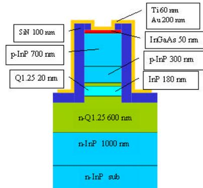
Figure 4: Layer stack of the phase shifters.
