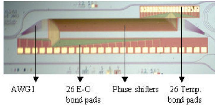
Figure 2: picture of the complete device and schematic description of its functionality.
