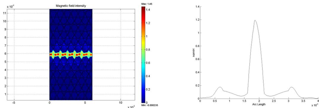
FIG. 3. Intensity distribution ( $|H_y|^2$ ) of a guided TE defect mode with normalized frequency 0.466. Left panel: surface plot; Right panel: cross-sectional view.
