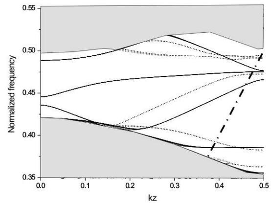
FIG. 2. Zoom-in of the projected band diagram (see text for structure details); grey areas are modes allowed in the bulk PCS and the white area is the photonic bandgap; TE and TM gap-guided modes are represented by continuous and dotted lines, respectively; the thick dash-dotted line is the light line of the air claddings.
