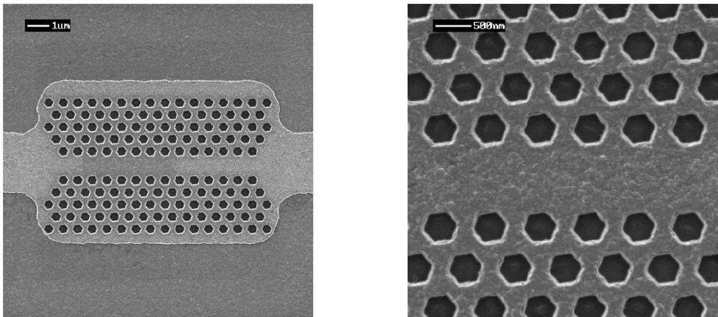
FIG. 4 Left panel: FIB-etched hexagonal-type photonic crystal pattern, aligned with waveguide pattern defined by conventional lithography in chromium. Right panel: detailed view.
