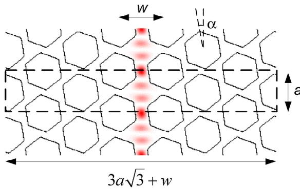
FIG. 1. Intensity distribution ( $|H_y|^2$ ) of well-confined guided TE defect mode (normalized frequency 0.466 at  $k_z = 0.5$ ) in hexagonal-type PCS. The supercell used for calculation is shown by the dashed contour.
