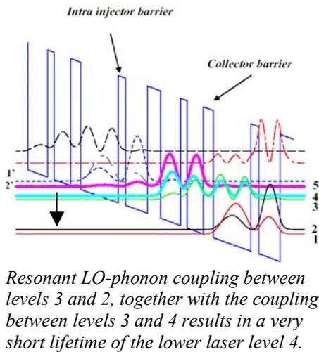
Fig. 2. Design of a 2.7 THz QCL based on LO-phonon depletion of the lower laser level (4). [7]
