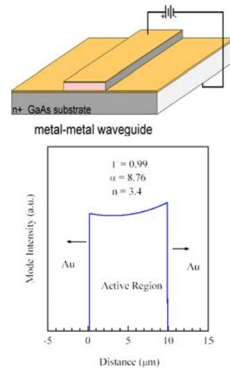
Fig. 4. Shape of the “metal-metal” waveguide and the optical mode profile for the QCL design shown in Fig. 2
