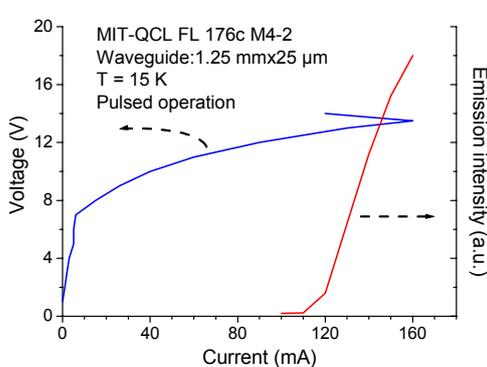
Fig. 5. I-V and L-I characteristics of 2.8 THz QCL with 1.25 mm x 25  $\mu\text{m}$  cavity dimensions.
