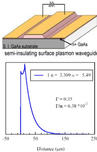
Fig.3 Shape of a “surface plasmon” waveguide and the optical mode profile for the QCL design shown in Fig. 2
