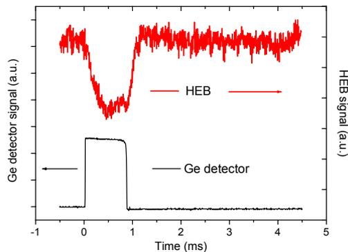
Fig. 10. Current response of the HEB (upper curve) and response of the Ge detector (lower curve) on the long pulsed 2.8 THz QCL
