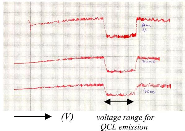
Fig. 11. Current response of the HEB detector as a function of driving voltage (current) of QCL in pulsed operation for different pulse duty cycles.
