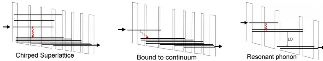
Fig. 1. Three different types of basic level schemes used for THz QCL's.
