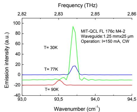
Fig. 6. Temperature dependence of emission spectrum of 25  $\mu\text{m}$  wide cavity sample.
