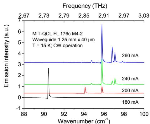
Fig. 7. Current dependence of emission spectrum of 40  $\mu\text{m}$  wide cavity sample.
