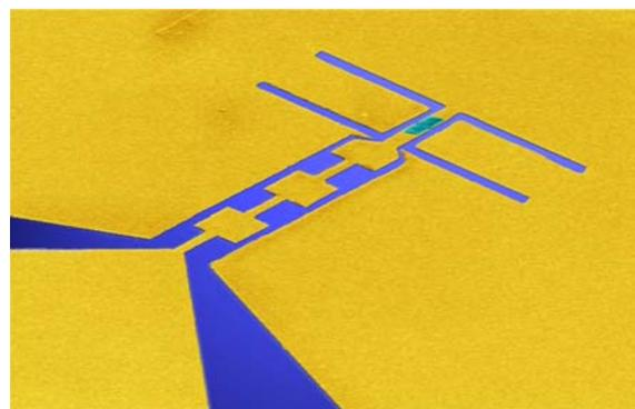
Fig. 8 Photo of the antenna coupled Hot Electron Bolometer
