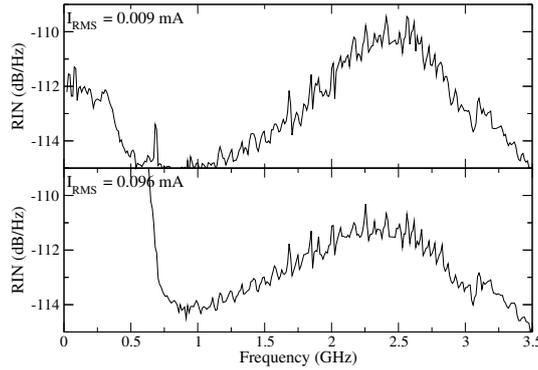
Figure 2: RIN spectra of the VCSEL under test at a constant current of 1.2 mA and at different carrier noise strengths.
