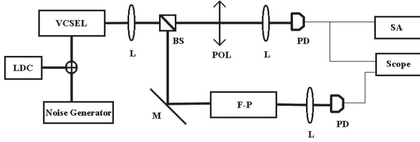
Figure 1: Scheme of the experimental set-up. VCSEL: thermally stabilized Vertical Cavity Surface Emitting Laser; L: collimating lens; BS: beam-splitter; POL: polarizer; M: mirror; PD: photodiode; FP: Fabry-Perot analyzer; LDC: laser diode controller; SA: spectrum analyser.
