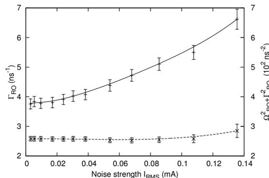
Figure 3: The relaxation oscillation damping rate  $\Gamma_{RO}$  (full) and  $\Omega_{RO}^2 + \Gamma_{RO}^2$  (dashed) as a function of the noise strength at a bias current of 1.2 mA.
