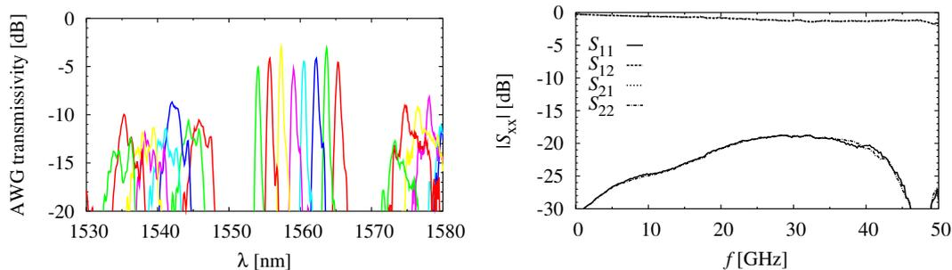
Figure 2: Measured chirped AWG passbands (left) and measured small-signal  $S$ -parameters of a CPW feed line with a length of 1.4 mm (right).
