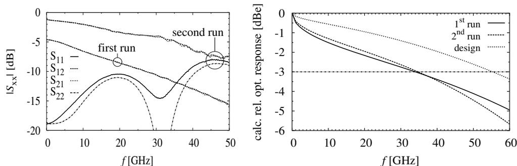
Figure 3: Measured  $S$ -parameters of a modulator with a phase-shifter length of 2 mm (left) and calculated bandwidth extracted from  $S$ -parameters measurements (right).
