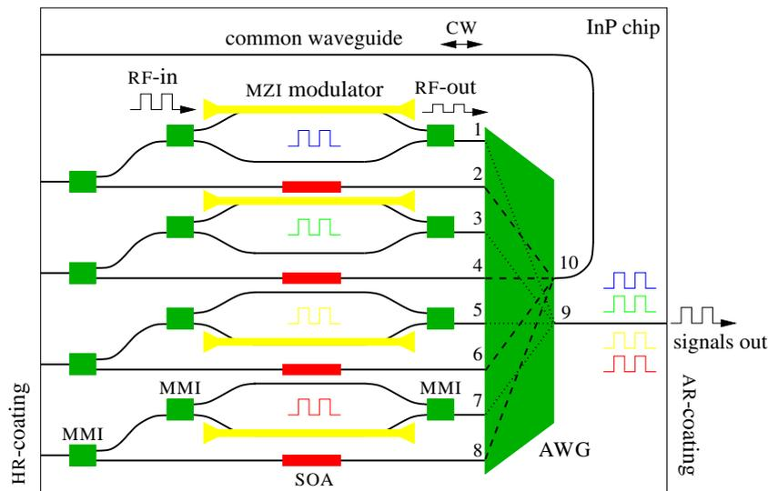
Figure 1: Schematic of the  $4\text{-}\lambda$  multiwavelength laser integrated with four modulators.
