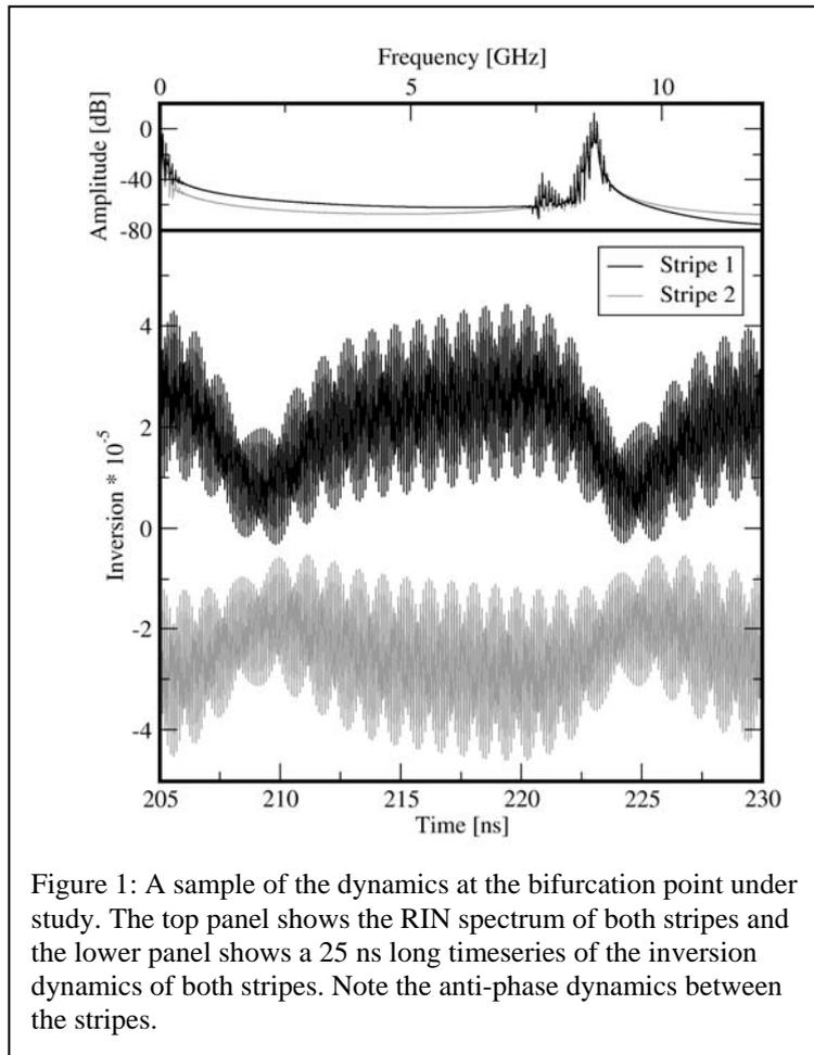
Figure 1: A sample of the dynamics at the bifurcation point under study. The top panel shows the RIN spectrum of both stripes and the lower panel shows a 25 ns long timeseries of the inversion dynamics of both stripes. Note the anti-phase dynamics between the stripes.
