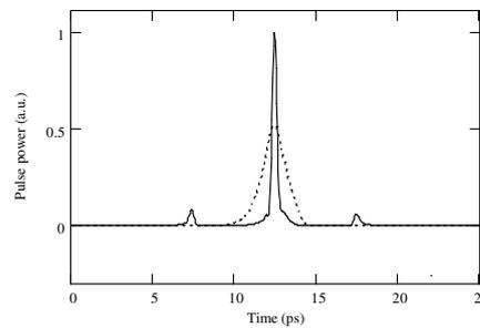
Fig. 4. Simulated optical pulse before (dotted) and after (solid) compression by the AWG-pair configuration of Fig. 3. The simulation is done using  $I=200\text{mA}$ . The AWG-pair dispersion is  $-0.1\text{ps}^2$ . The compressed pulsewidth is 300fs. 20 delay lines are used.
