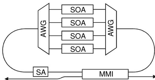
Fig. 5. Intracavity pulse shaping, using four SOAs of  $500\mu\text{m}$ . The AWGs have a channel spacing of 200GHz. A 40GHz cavity is assumed and  $L_{SA}=50\mu\text{m}$ .
