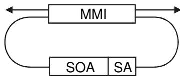
Fig. 1. 40GHz mode-locked ring laser configuration based on [9]. For simulation purposes the SOA and SA lengths are respectively  $L_{\text{SOA}}=500\mu\text{m}$  and  $L_{\text{SA}}=50\mu\text{m}$ . The MMI is a 50/50 splitter.
