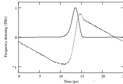
Fig. 2. Pulse power (solid, a.u.) and chirp profile (dotted) using  $I=130\text{mA}$ . The cavity dispersion is  $0.01\text{ps}^2$ .
