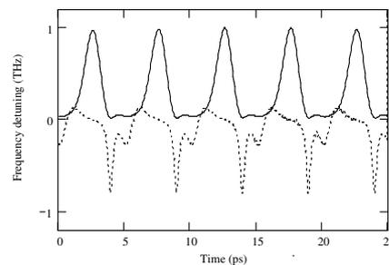
Fig. 6. Simulated output pulse power (solid, a.u.) and chirp (dotted) from the laser configuration of Fig. 5.
