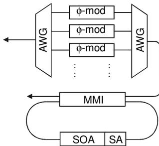
Fig. 3. AWG-pair with tunable delay lines added to the output of the ring laser of Fig. 1. The AWGs have a 200GHz channel spacing and a Gaussian transmission. The phase modulators are indicated by  $\Delta\phi$ . The dots indicate the variable number of phase modulators.
