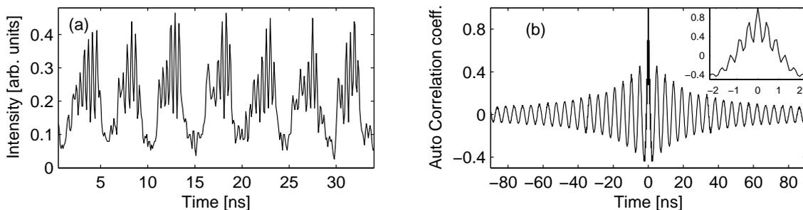
Figure 2: In (a) a typical time trace of a laser intensity in pulse packages regime and in (b) its auto-correlation function. The inset of plot (b) illustrates the regularity of the PP dynamics at the multiples of the delay.
