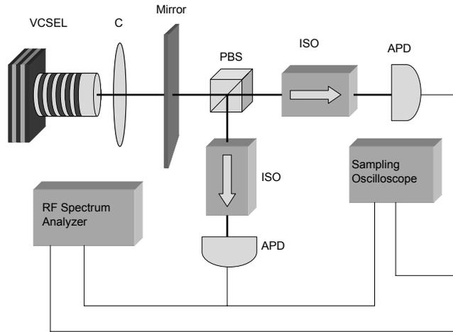
Figure 1: Schematic illustration of the experimental setup: C is the collimating lens, PBS, polarizing beam splitter, ISO, optical isolators, APD, avalanche photodiodes.
