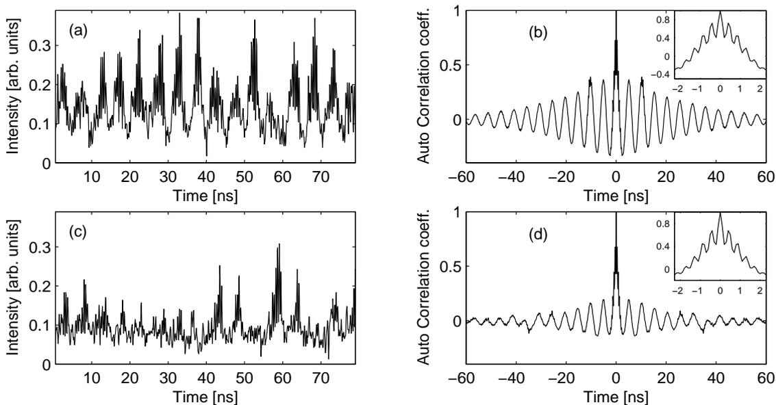
Figure 3: Polarization resolved dynamics of a VCSEL in PP regime. In (a) and (c) we plot time traces of a x-(y) polarized mode respectively. In (b) and (d) we plot the corresponding auto-correlation functions of the two polarization modes.
