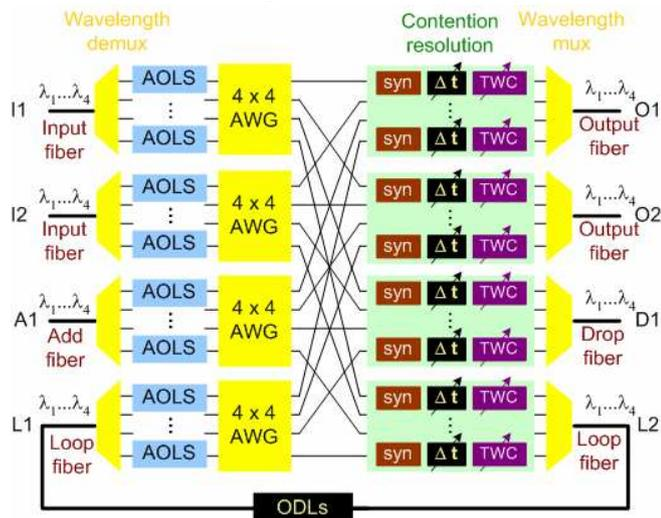
Fig. 2. A 2x2 AOLS WDM packet switch (AOLS: all-optical label swapper, AWG: arrayed waveguide grating, Demux: optical demultiplexer, Mux: optical multiplexer, ODLs: optical delay lines, syn: synchronization, TWC: tunable wavelength converter)
