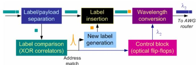
Fig. 3. AOLS original: subsystems block diagram
