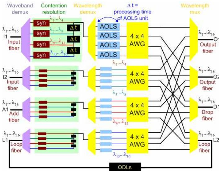
Fig. 5. Regular AOLS packet switch schematic configuration with contention resolution
