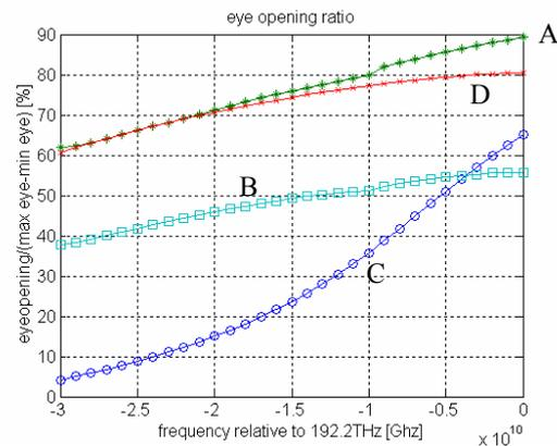
Figure 5 eye opening ratio (flat-top filter)
