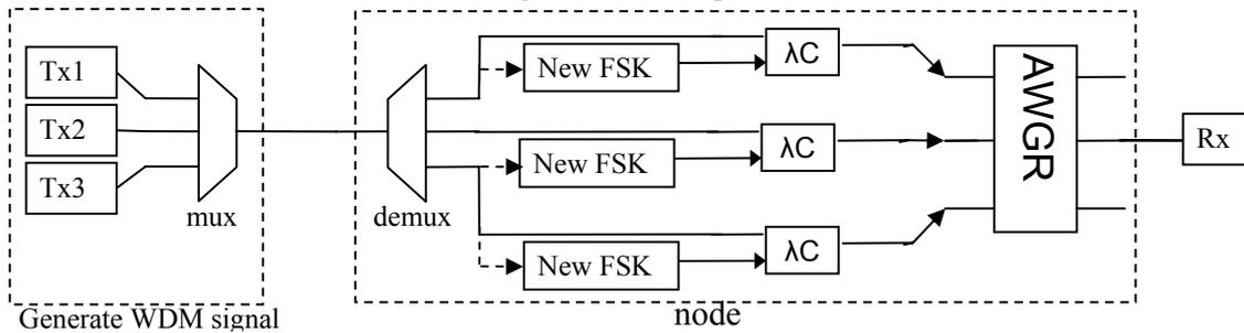
Figure 1 simulation architecture of core node under study ( $\lambda C$  : wavelength converter)
