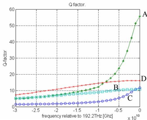
Figure 4 Q-factor (flat-top filter)
