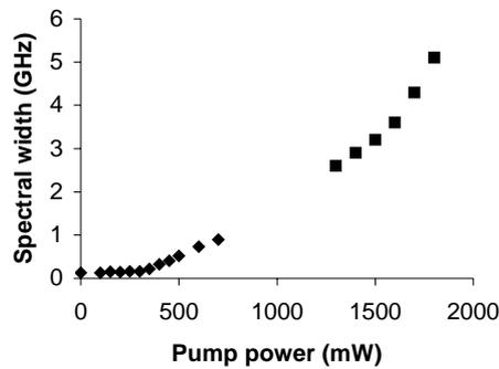
Fig. 2: Spectral broadening of the signal at the output of the RFA measured with the FP ◆ and with the OSA ■
