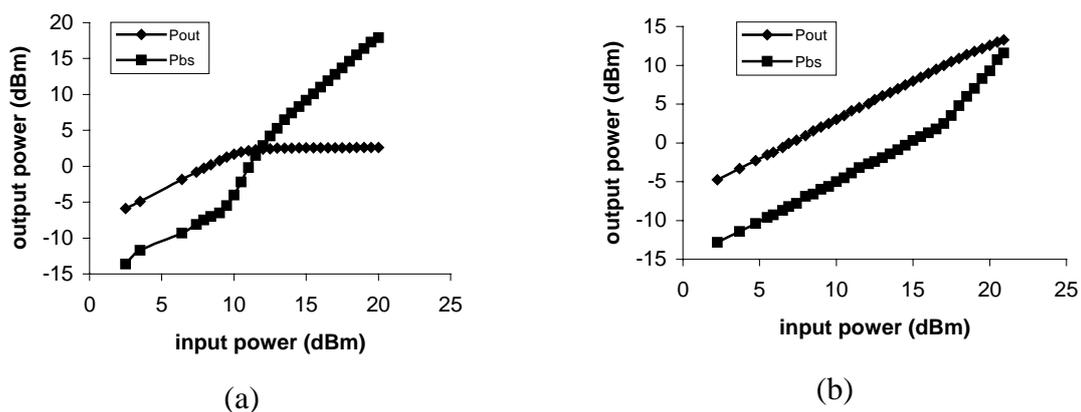
Fig. 3: Output power ( $P_{out}$ ) and SBS backscattered power ( $P_{bs}$ ) as a function of the input power in the case of (a) a narrow bandwidth signal and (b) a signal spectrally broadened by XPM
