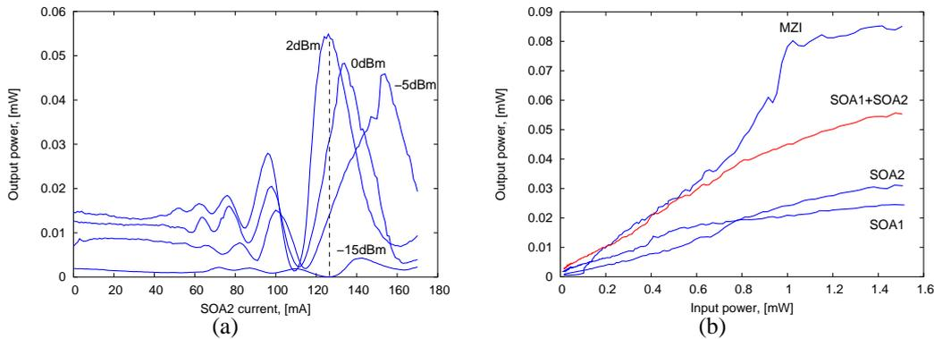
Figure 3: Measured interference curves (a) and transmission curves (b). Input and output power are the ones in the fiber. The fiber-to-chip coupling losses are not taken here into account.
