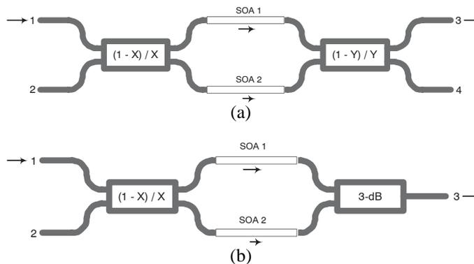
Figure 1: Schematics of MZI-based switches with unequal power distribution:  $2 \times 2$  (a) and  $2 \times 1$  (b).
