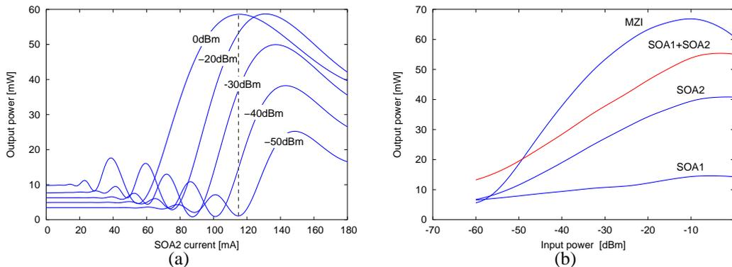
Figure 2: Calculated interference curves for input powers -50 dBm - 0 dBm (a) and transmission curves for only SOA1, SOA2, sum of these two and the full MZI (b).
