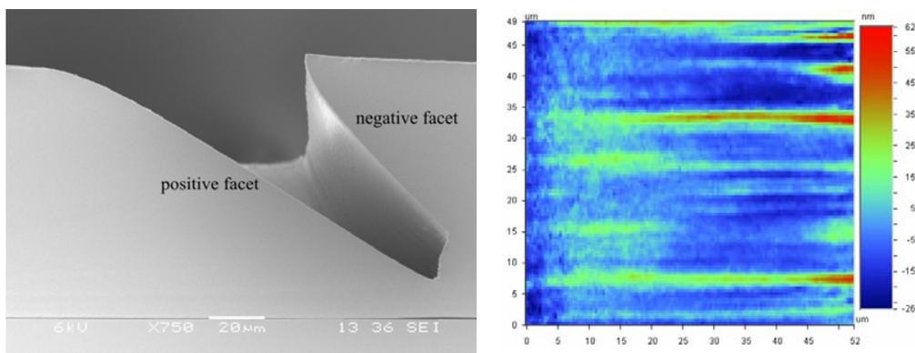
Fig.2. Micromirror fabricated in ORMOCER<sup>®</sup> using excimer laser ablation. Left: SEM picture of cross section. Right: WYKO plot to analyze surface roughness
