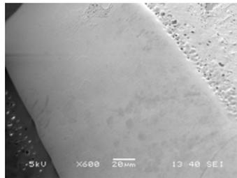
Fig.4. SEM picture of a micromirror fabricated in a 100 μm thick glass sheet using CO<sub>2</sub> laser ablation
