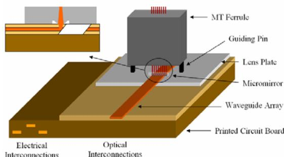
Fig.1. Cross-sectional schematic diagram of the optical interconnection
