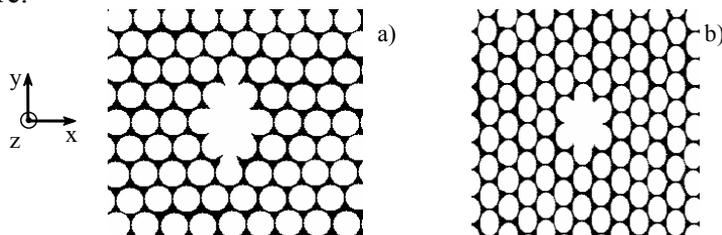
**Fig 1.** Cross-section of the PCF: **a)** based on the hexagonal lattice with the elliptical shape of the core; **b)** based on the squeezed hexagonal lattice.
