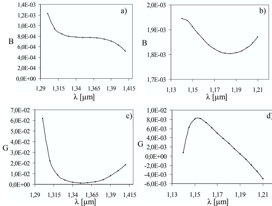
**Fig. 3** Phase birefringence  $B$ , and group birefringence  $G$  in the function of wavelength. **a)**  $B$  for the PCF from Fig. 1a; **b)**  $B$  for the PCF from Fig. 1b; **c)**  $G$  for the PCF from Fig. 1a; **d)**  $G$  for the PCF from Fig. 1b.
