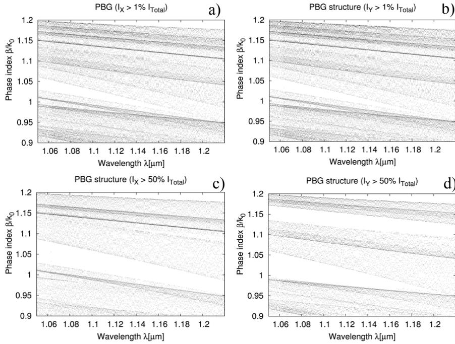
**Fig. 2.** The photonic bandgap of the squeezed air-silica lattice from Fig 1.b. vs. wavelength. The plotted modes contain **a)** over 1% of energy in the X-polarization; **b)** over 1% of energy in the Y-polarization; **c)** over 50% of energy in the X-polarization; **d)** over 50% of energy in the Y-polarization.
