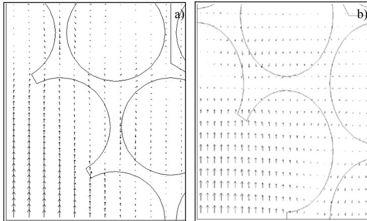
**Fig. 4.** Electric field distribution of the Y-polarized mode calculated over one quarter of the fiber's cross-section: **a)** for the PCF from Fig. 1a, at  $1.3\mu\text{m}$ ; **b)** for the PCF from Fig. 1b at  $1.13\mu\text{m}$ .
