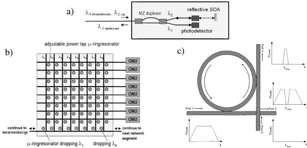
**Figure 2:** Optical network unit architecture (a), wavelength router schematic (b), micro ring resonator schematic (c).
