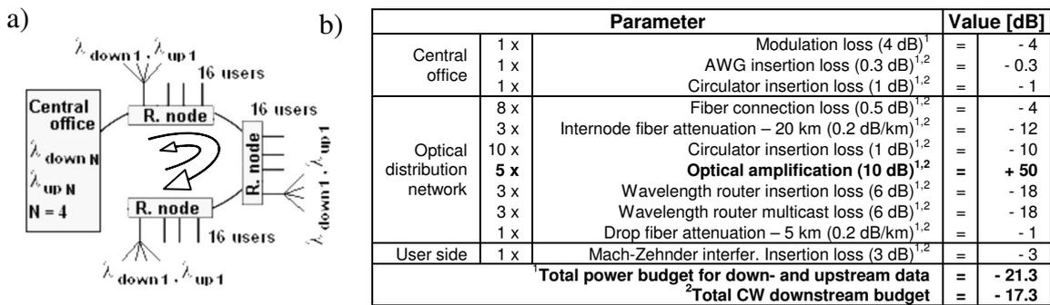
**Figure 3:** The longest light path definition (a) and the longest light path power budget for down- and upstream transmission (b).
