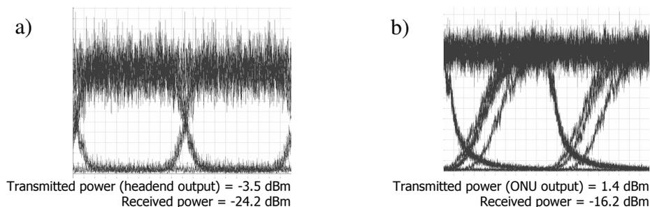
**Figure 4:** Eye diagrams of received downstream (a) and received upstream signals (b).
