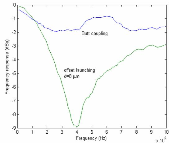
**Figure 4.** Measured frequency response of a 50/125  $\mu\text{m}$  GIMMF,  $L=750\text{m}$ .
