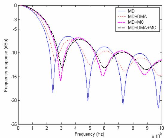
**Figure 2.** Influence of the differential mode attenuation and mode coupling. The index exponent  $\alpha=2.0$ . Other parameters are the same as used in Fig. 1. MD: modal delay, MC: mode coupling, DMA: differential mode attenuation.
