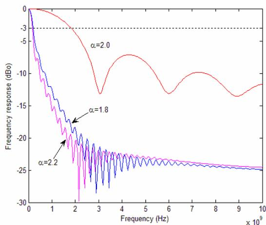
**Figure 1.** Frequency responses for a 2000-m-long fibre with  $\lambda_0=1300$  nm and index exponent  $\alpha=1.8$  2.0 and 2.2. The mode delay, differential mode attenuation and mode coupling are all included.
