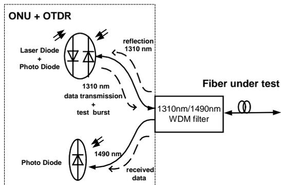
Figure 2: Proposed embedded OTDR for PON
