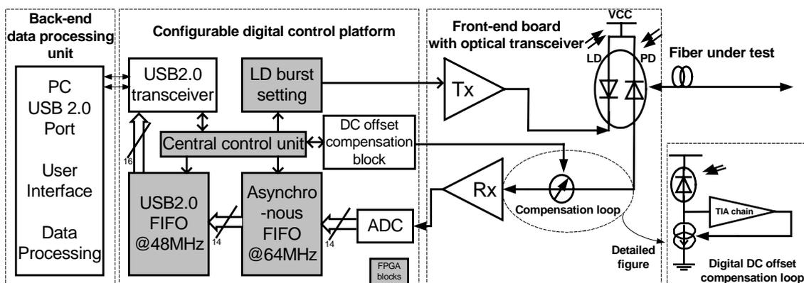
Figure 3: Proposed embedded OTDR experimental set-up
