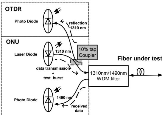
Figure 1: Current embedded OTDR for PON
