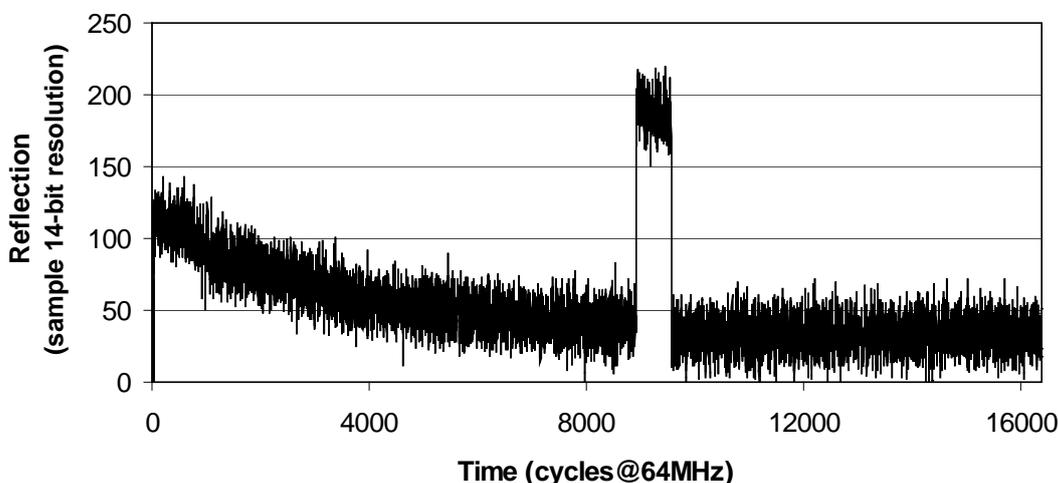
Figure 4: Embedded OTDR curve from proposed experimental set-up
