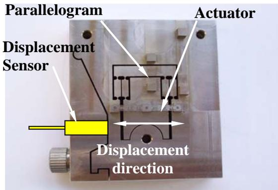
Figure 1. Parallelogram base and actuator.
