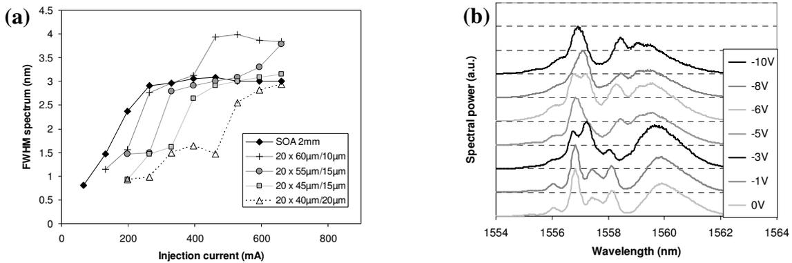
Fig. 3: (a) Measured spectral widths (FWHM) for different IRIS configurations with 20 SOA/SA pairs. The applied reverse bias on the SAs is  $-1V$ . The injection current is supplied by a pulsed source, using 300ns pulses and 1% duty cycle. (b) Normalized output pulse spectra after propagation through a configuration with short SAs ( $20 \times 60\mu\text{m}/10\mu\text{m}$ ), applying different reverse bias voltages.
