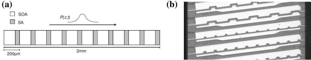
Fig. 1: (a) Schematic overview of the IRIS configuration used in the simulations. An input pulse (denoted by  $P(z,t)$ ) enters from the left side, entering an SOA and exiting from the right-hand side. The ratio of the SOA and SA length within the  $200\mu\text{m}$  section is varied. (b) Photograph of the realized devices, showing different configurations.
