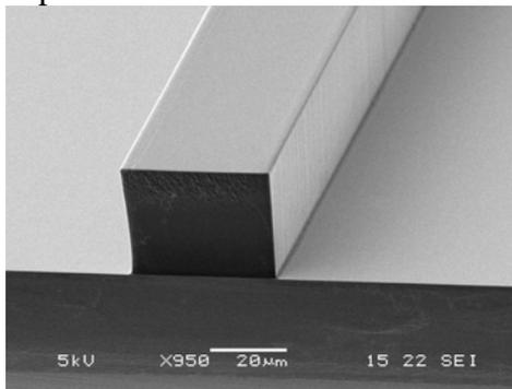
Fig. 2a. SEM picture of a CHEP-DGEBA-triol core.
