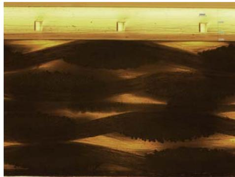
Fig. 2b. Microscope picture of embedded waveguides deposited onto a FR-4 PCB substrate; the fiberglass yarn is clearly visible.
