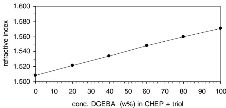
Fig. 1. Refractive index @ 850 nm of CHEP film waveguides as a function of DGEBA content.
