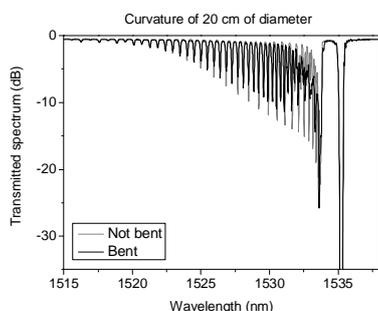
Figure 5. Effect of a curvature on the transmitted spectrum of a 3° TFBR.
