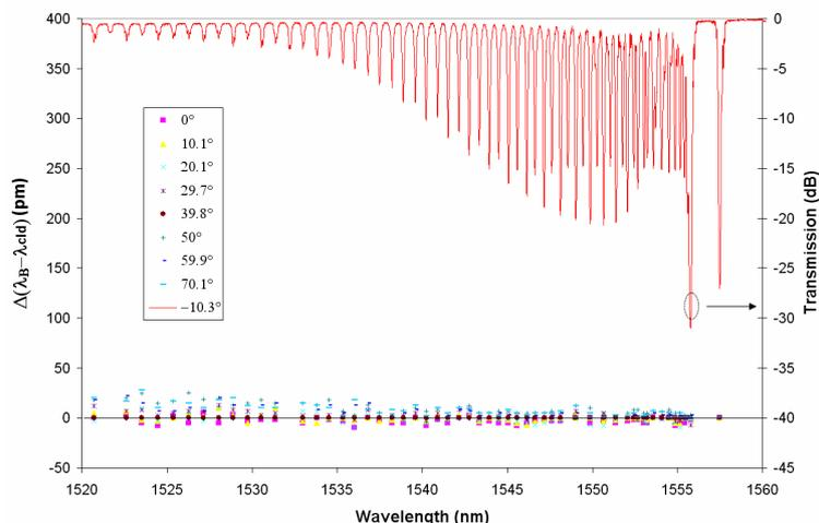
Figure 4. Transmitted spectrum of a 4° TFBR and differential wavelength shift due to temperature.
