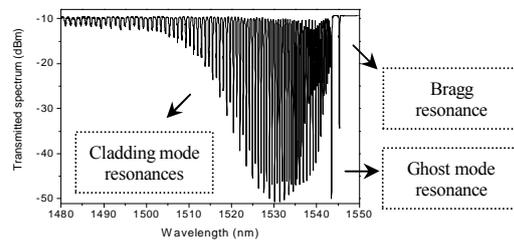
Figure 2. Transmitted spectrum of a 3° TFBG.
