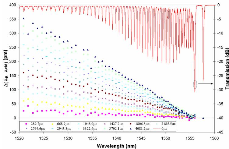
Figure 3. Transmitted spectrum of a 4° TFBG and differential wavelength shift due to strain changes.
