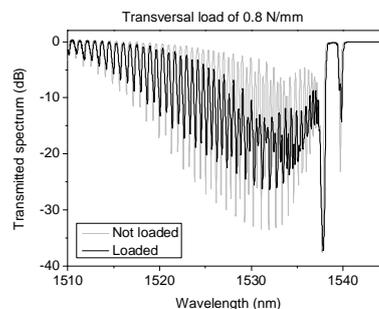
Figure 6. Effect of a transversal load on the transmitted spectrum of a 4° TFBR.
