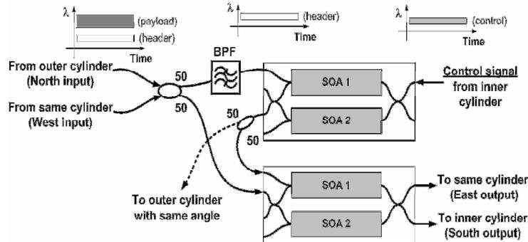
Fig. 1 Configuration of the proposed all-optical Data Vortex node employing MZI-SOA gates
