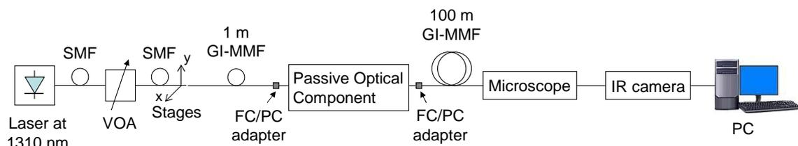
Figure 2: Experimental set-up for the investigation of the effect of passive optical components on the NFP of GI-MMF links.
