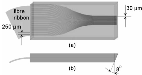
Fig.1 (a) Top view FSC, 16 fibers with 250  $\mu\text{m}$  interval spacing are converted to 30  $\mu\text{m}$  spaced intervals. (b) Side view FSC, the end facet is polished at an angle of 8°.
