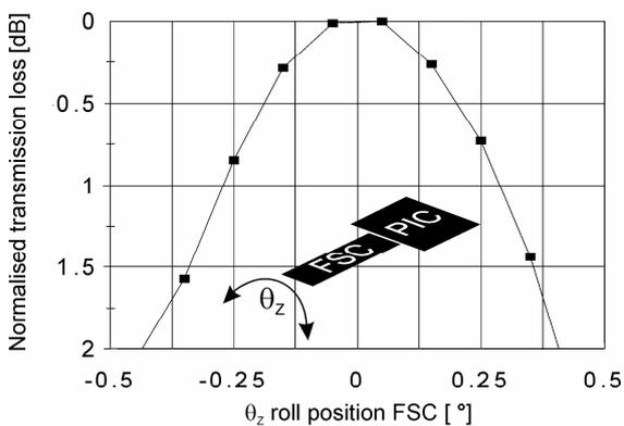
Fig. 6 Normalised additional transmission loss increment as a function of the rotational roll position of the FSC compared with the chip facet.
