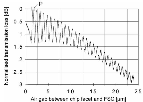
Fig. 5 Oscillating interference phenomenon because of the air gab between the FSC and chip fact. All measurements are registered at point P.
