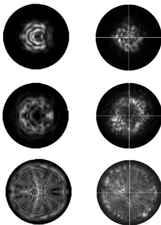
Figure 1: Simulations (left) and measurements (right) at  $z = 1\text{m}$ . Upper:  $ro=13\mu\text{m}$ ; centre:  $ro=13\mu\text{m}$  and  $ao=6.5^\circ$ ; bottom:  $ro=26\mu\text{m}$ .
