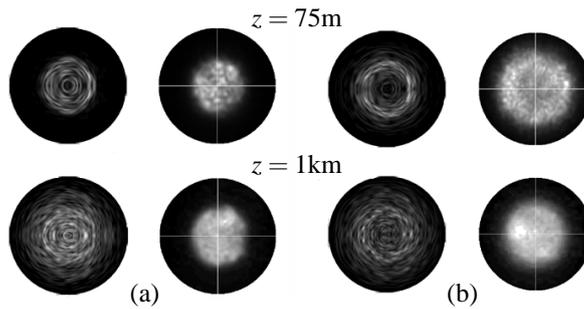
Figure 2: Simulations (left) and measurements (right) at  $z = 75\text{m}$  and  $z = 1\text{km}$  (a): for  $ro=13\mu\text{m}$ ; (b): for  $ro=13\mu\text{m}$  and  $ao=6.5^\circ$ .
