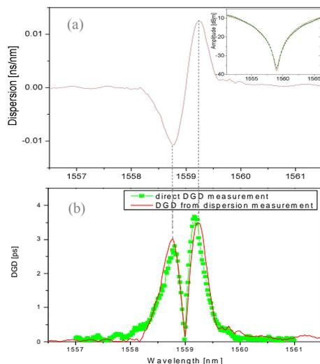
Fig. 1. LPG chromatic dispersion (a) and DGD (b); amplitude response (in the inset in (a)).
