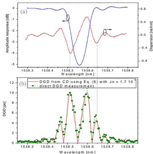
Fig. 2. FBG response: amplitude and CD (a) and DGD (b)
