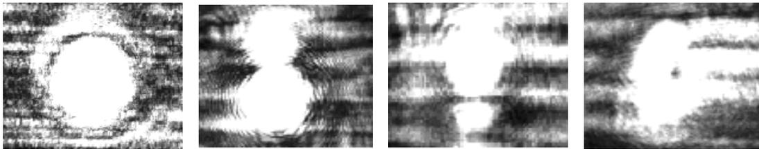
Fig. 1. Near-field mode profiles of fs-laser written waveguides. a) fundamental mode b) 1<sup>st</sup> order mode, c) 2<sup>nd</sup> order mode, d) 'donut' mode
