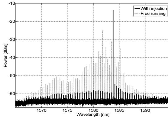
Figure 3 – Optical spectrum of the ring laser with and without co-propagating injection seed showing single mode operation with 40dB side mode suppression
