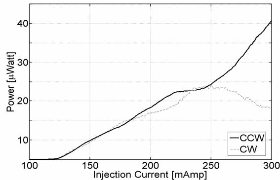
Figure 2 - Output Power of both counter propagating modes in the ring as a function of current injection
