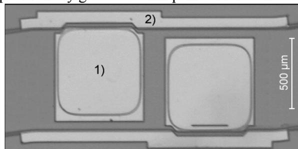
Figure 1 - Top view of two QD ring lasers with two separate electrical contacts; 1) For the ring and the directional couplers and 2) For the output waveguides.
