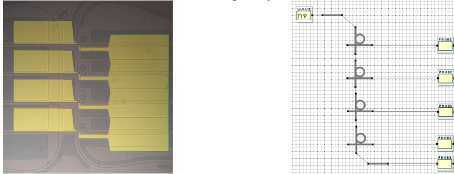
Figure 6. (Left) Microscope image of fabricated OADM. (Right) Implementation in Aurora.
