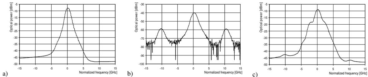
Fig. 5: RSOA output spectrum when no RBS or bias dithering is present a), spectrum of the backscattered power b), RSOA output spectrum when RBS and bias dithering are present c)
