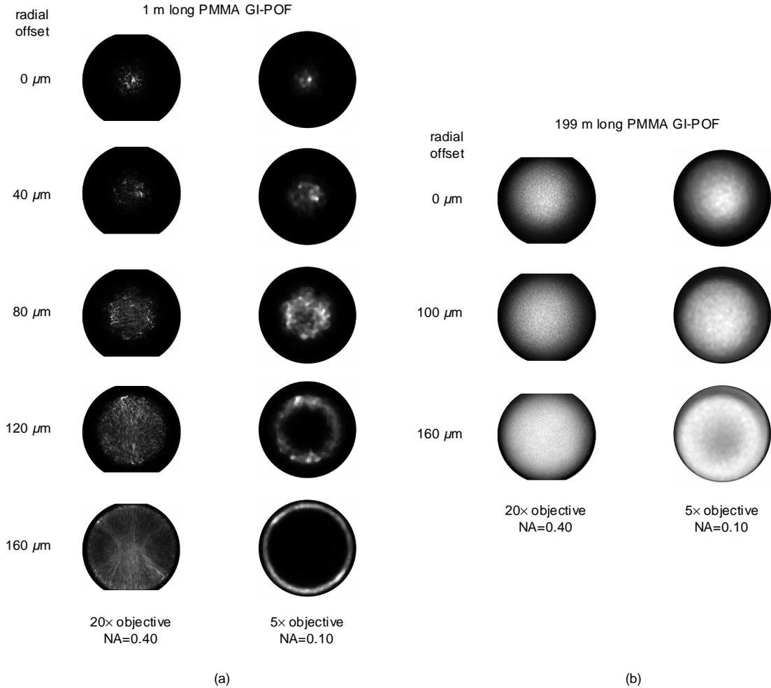
Figure 1: Observed NFPs at the output end of a (a) 1 m (b) 199 m long PMMA-based GI-POF under selective excitation with an SMF, at 635 nm wavelength. Each row corresponds to a different radial offset of the input SMF and each column to a different microscope objective. The 20 $\times$  magnified core exceeds the dimensions of the CCD camera. Mode-selective spatial filtering is achieved with the 5 $\times$ , 0.10-NA microscope objective [6].
