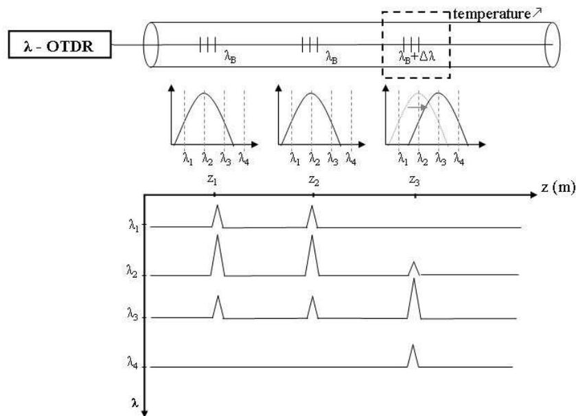
Figure 1: Sensor principle: when the  $\lambda$ -OTDR emitted wavelength is included within the reflection spectrum of one of the gratings, the OTDR trace contains a reflection peak located at this FBG's position. For each FBG, the reflection spectrum is rebuilt from the different magnitudes of the reflection peaks corresponding to each wavelength emitted by the  $\lambda$ -OTDR
