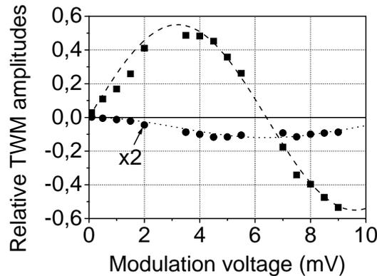
Fig.3. Experimental dependences of relative amplitudes of odd (squares) and even (circles) TWM signal components on  $U_{\text{mod}}$  at  $P_{\text{in}} = 5 \text{ mW}$ . Solid lines present fitting by expected theoretical dependences.
