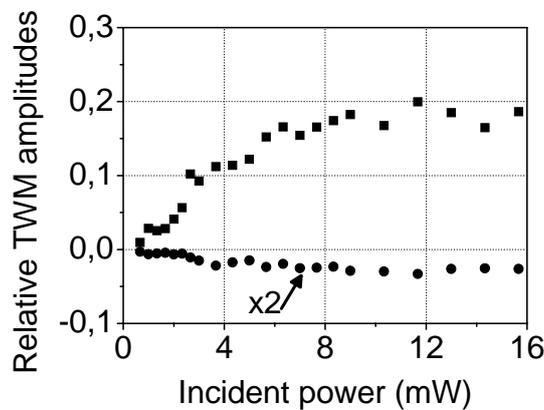
Fig.4. Experimental dependence of relative amplitude of the of odd (squares) and even (circles) TWM response components on input light power  $P_{\text{in}}$  ( $U_{\text{mod}} = 1 \text{ V}_{p-p}$ ).
