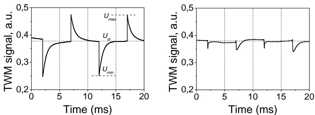
Fig.2. Typical transient TWM signals observed in under rectangular modulation with amplitude  $U_{mod} \approx U_{\pi/2}$  (left) and  $U_{mod} \approx U_{\pi}$  (right) with averaging over 512 oscilloscope traces.
