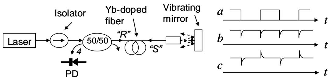
Fig.1. Experimental set up utilized in experiments on transient TWM in Yb-doped fibers and profiles of the rectangular modulating signal (a), and typical transient TWM responses expected for unshifted amplitude (b) and phase (c) dynamic gratings.
