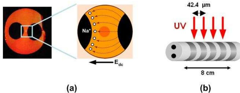
Fig.1: (a) Cross section image of a twin-hole silica fibre. The enlargement on the core region shows the drift of the Na<sup>+</sup> ions as a result of the process of thermal poling. (b) UV erasure of the thermally poled silica fibre to achieve quasi-phase matching condition during parametric fluorescence.
