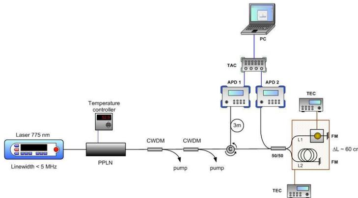
Fig.4: Experiment setup leading to two photon interferences in an unbalanced Michelson interferometer. See Fig.2 for components enumeration.
