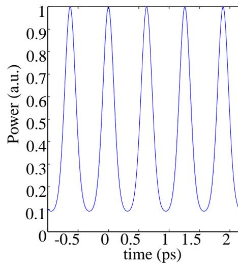
Figure 3: Pulse train generated at the output of the cavity (numerical results).
