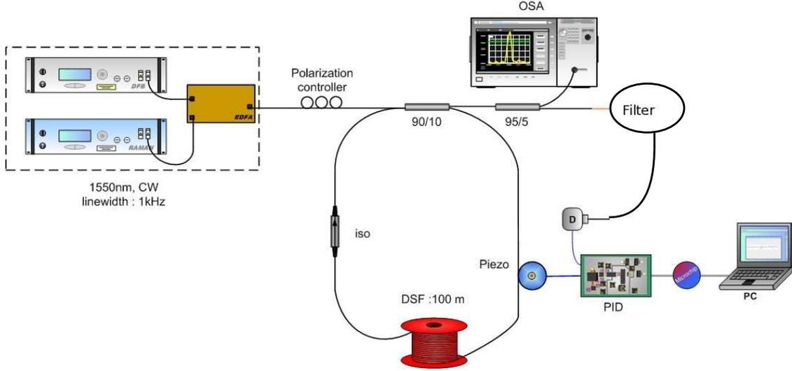
Figure 1: Experimental setup. DSF length 100 m, SMF28 length 0.8 m (inside coupler and isolator). The zero dispersion wavelength of the DSF was measured at 1550.6 nm.
