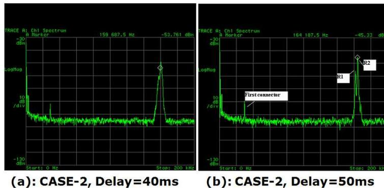
Figure 4: Comparison between two different time gate position. a) delay = 40 ms, reflections R1 and R2 are not resolved, b) delay = 50 ms, reflections R1 and R2 are clearly resolved
