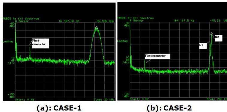
Figure 3: Comparison between two different sweep rates. a)  $\gamma_v = 1.25$  THz/s, reflections R1 and R2 are not resolved, b)  $\gamma_v = 12.5$  THz/s, reflections R1 and R2 are clearly resolved
