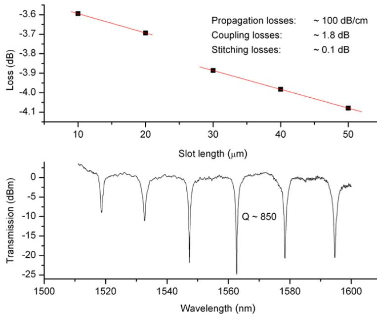
Figure 2: Top: transmission measurements of slots etched in a straight silicon waveguide yield a propagation loss of 100 dB/cm. Bottom: transmission spectrum of slot racetrack resonator. We have measured a Q value of about 850 and an extinction ratio of 25 dB.
