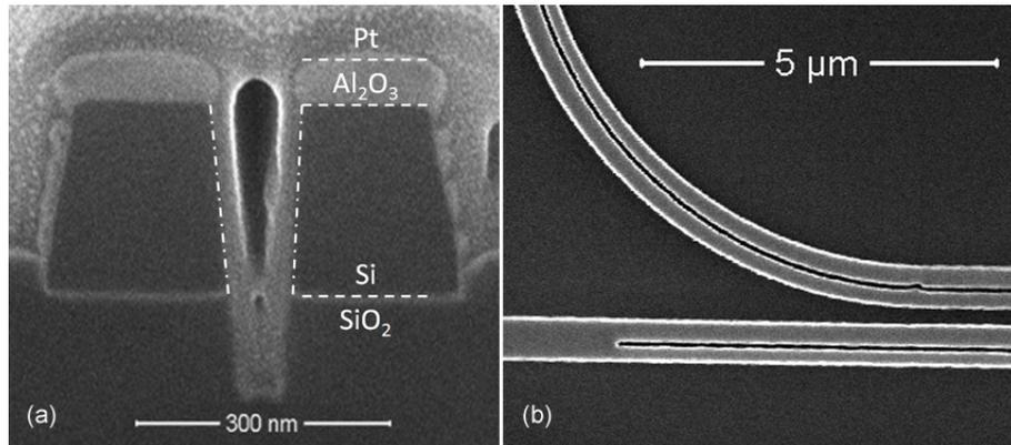
Figure 1: Cross-sectional micrograph (after Pt deposition) (a) and top view (b) of a FIB etched slot in waveguide and racetrack resonator.
