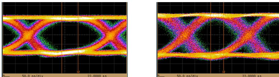
Figure 3: Eye diagrams for 3 Gbit/s (left) and 4 Gbit/s (right) with  $-12\ \text{dBm}$  input optical power.
