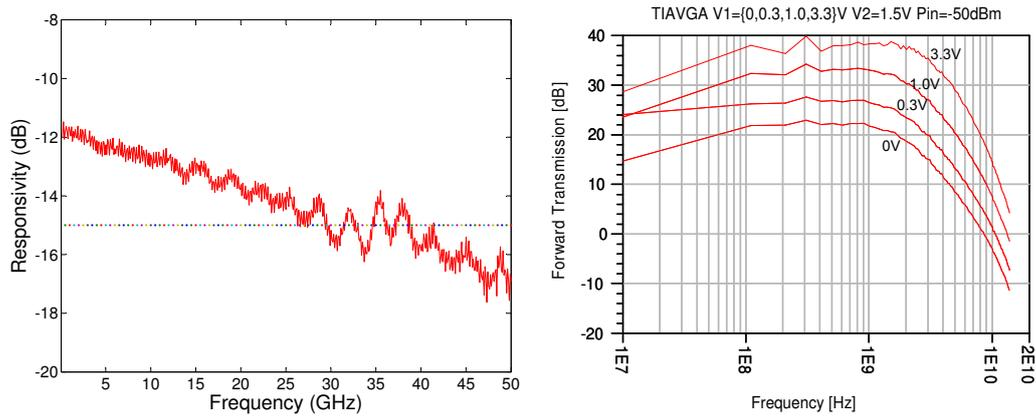
Figure 2: Left: Measured bandwidth and responsivity of  $30\ \mu\text{m}$  long InP based photodetector. Right: the measured bandwidth of SiGe amplifier at different gain control voltages.
