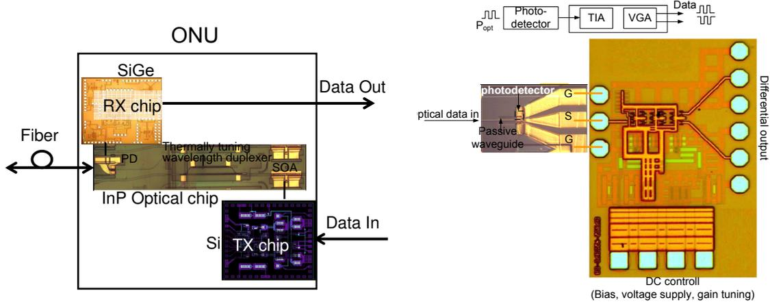
Figure 1: Left: Colorless ONU building blocks with three chips (sizes are not in scale). Right: Block functionality diagram of the photoreceiver and the photograph of the fabricated photoreceiver consisting of an InP-photodetector and a SiGe amplifier connected with bonding wires.
