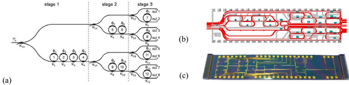
Figure 3. OBFN binary-tree topology (a), layout (b) and picture (c).
