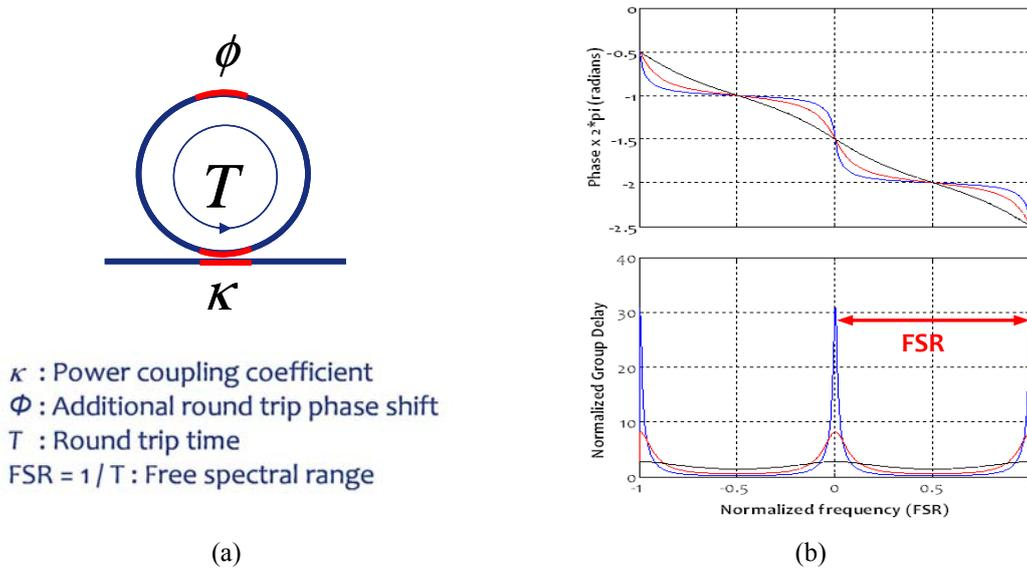
Figure 1. Optical ring resonator (ORR) used as true time delay (TTD) unit. Tuning parameters (a) and spectral characteristics (b).
