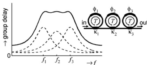
Figure 2. Cascaded optical ring resonators (ORR) are used to increase the band of the TTD unit.
