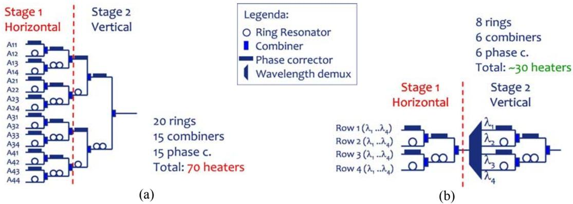
Figure 4. Comparison between the traditional binary-tree (a) and the multi-wavelength, multiple signal path OBFN (b), for a 4x4 planar array. Note the dramatic reduction in the number of heaters required.
