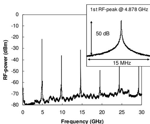
Fig. 3 RHS output RF-spectrum obtained with a ring injection current of 820 mA and an SA bias voltage of -1 V. The output waveguide current is 150 mA. Inset: Detailed view of the spectrum around the first RF-peak.
