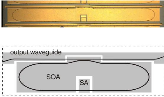
Fig. 1 (top) Picture of the realized devices. (bottom) Schematic overview of the QD ring MLLD, showing the separate contacts (grey) for the SOA, SA and output waveguide. The waveguides are indicated by the black line.
