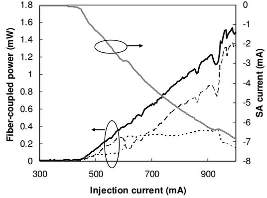
Fig. 2 Measured fiber-coupled output power for the LHS-output ( $\times 10^3$ , dashed) and RHS-output (dotted) and the calculated summation of both (solid black). The reverse bias current generated in the SA is also given (solid grey).  $V_{\text{SA}} = -1 \text{ V}$ .
