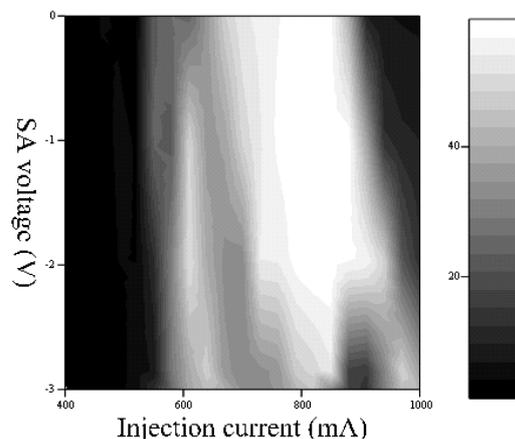
Fig. 4 RHS output RF-peak heights (dB-scale) as a function of SA bias voltage and ring injection current. The same settings as in Fig. 3 are used.
