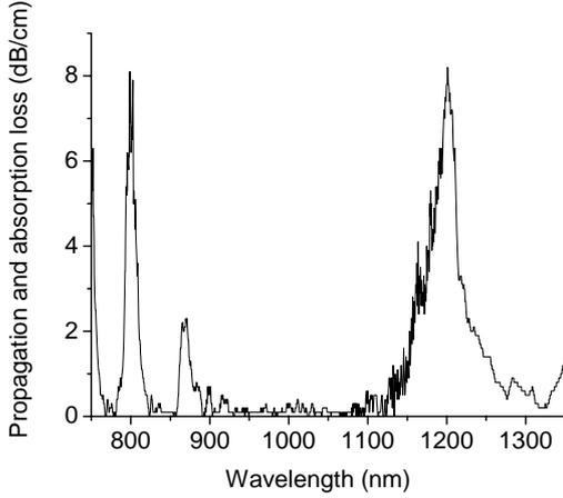
Fig. 1. Loss spectrum of  $\text{Nd}^{3+}$ -doped 6-FDA/epoxy
