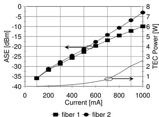
Fig. 6 ASE power as a function of the driving current through the SOA measured at 10 °C and reduced electrical power to control the TEC by active cooling of the mounting plate.
