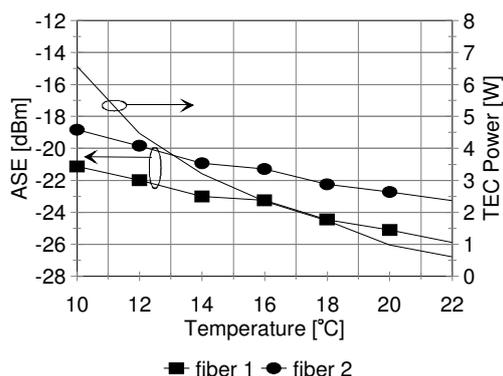
Fig. 5 ASE power as a function of the chip temperature and electrical power to control the TEC. The driving current through the SOA is 500 mA.
