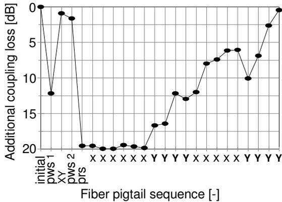
Fig. 3. Measured normalized received optical power of fiber 1 as a result of the following actions: after the first weld joint (pws1), again optimization of the fiber in the xy-plane, after the second weld joint (pws2), and subsequently after releasing the alignment tool (prs). In the next sequence, the fiber is aligned to the initial position by using laser-support adjustment.
