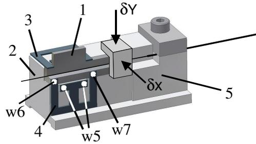
Fig. 1 Schematic presentation of the fiber-subassembly. The fiber tip (2) can be laser-adjusted in the x- and y-direction using both tuning frames (3) and (4).
