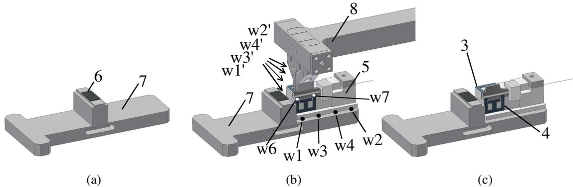
Fig. 2 Sequence of the pigtail procedure: (a) Chip (6) is bonded onto a carrier (7). (b) The fiber-subassembly (5) is aligned and welded onto the carrier (7) using weld sequence (w1) and (w1'), (w2) and (w2'), (w3) and (w3'), (w4) and (w4') simultaneously. Next, the height of the fiber is fixed by weld joints (w6) and (w7). (c) After removing the pneumatic alignment tool (8) the final fine alignment can be executed at the tuning frames (3) and (4) using laser-adjusting.
