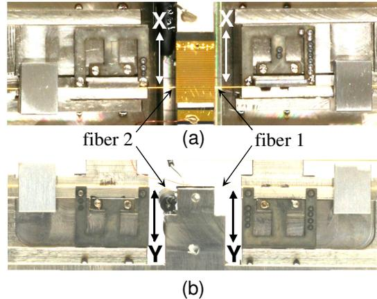
Fig. 4. (a) Top view of the fiber-supports and tuning frames to adjust the fibers in the x-direction. (b) Side view of the tuning frames to adjust the fibers in the y-direction. Fiber 1 is laser-adjusted 19 times, while fiber 2 was only laser-adjusted five times to re-adjust the fiber back to the initial position.
