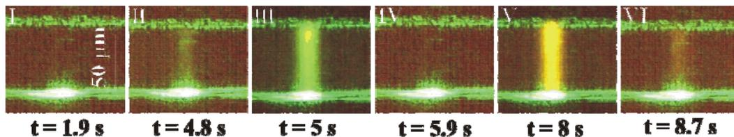
Fig.2. Passage of fluorescent dyes Rhodamine-6G and Rhodamine-B during CE separation in a MF channel, across an excitation WG
