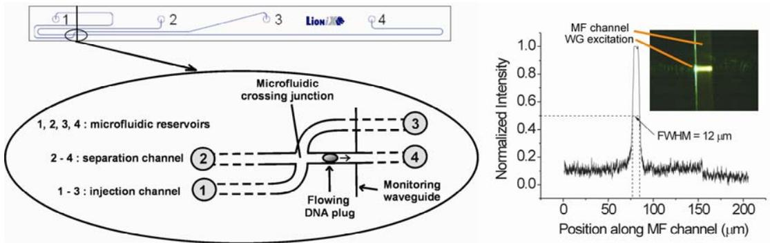
Fig.1. Layout of the MF chip with an integrated optical WG, schematic of the MF chip, with the fluorescent plug passage monitored by the integrated WG, and the resulting distribution of fluorescence intensity along the MF channel
