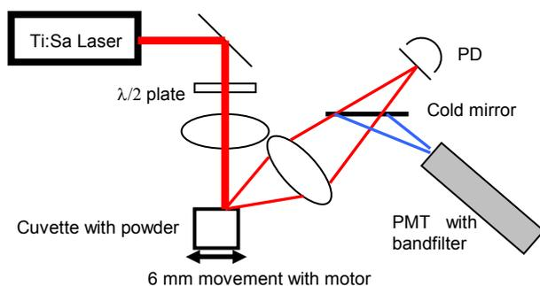
**Fig. 1:** Overview of the experimental setup.
