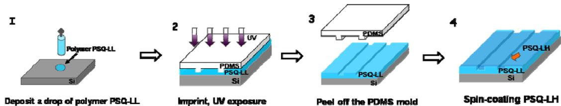
Fig.2 Fabrication process flow of the polymer waveguides
