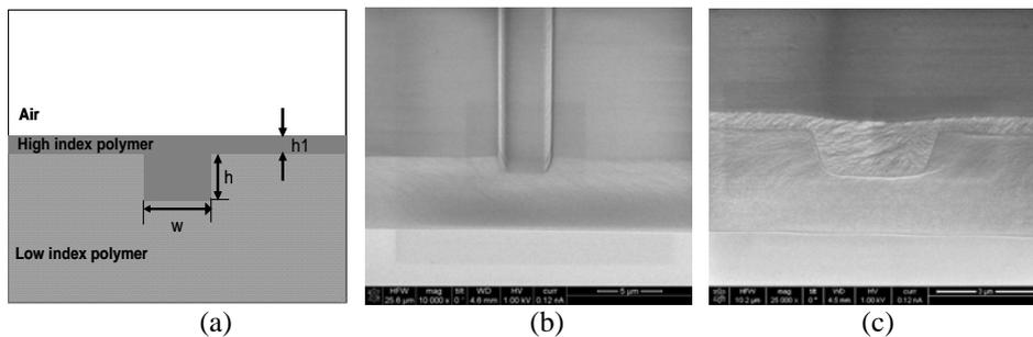
Fig.1 (a) The cross-section of the waveguide (b) SEM picture of the imprinted low index layer (c) SEM picture of waveguide cross-section (after spin-coating the high index layer)
