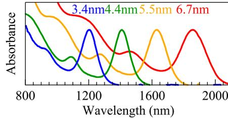
Figure 1: Absorbance spectra of different Q-PbSe suspensions. A blue shift of the transitions with decreasing Q-PbSe size is observed.
