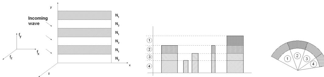
Figure 1: Scattering by a horizontal set of N-layers, a telegrapher's wave- and an insect's eye type of surface. The shaded parts can have different values for the refractive index.
