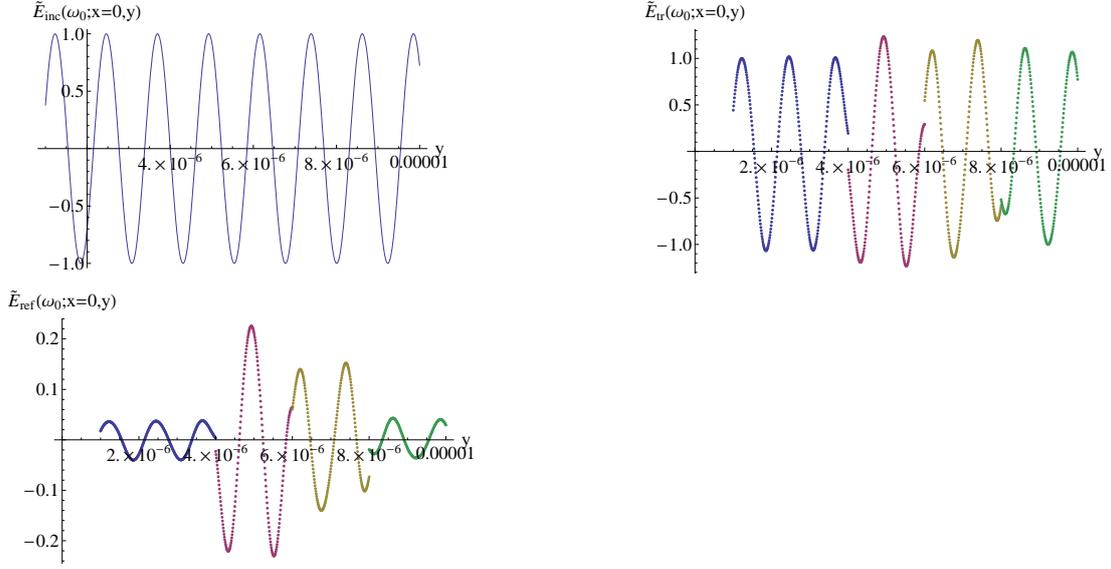
Figure 3: Distributions of the incoming, transmitted and reflected fields at the interface at  $x = 0$  between a homogeneous medium to the left and a horizontal set of two layers to the right.
