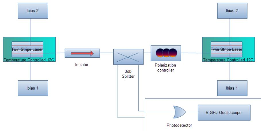
**Figure 3** Synchronization set-up.
