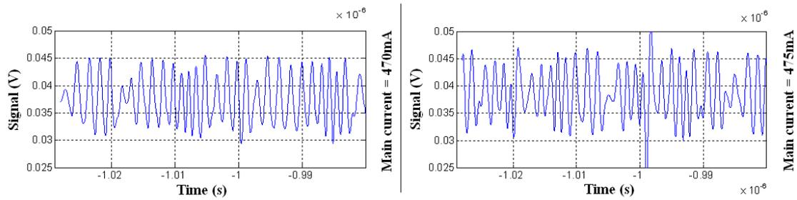
**Figure 2** Time responses of the twin stripe corresponding to a fix value of  $I_{\text{neigh}}$  (400mA) and 2 different values of  $I_{\text{main}}$ .
