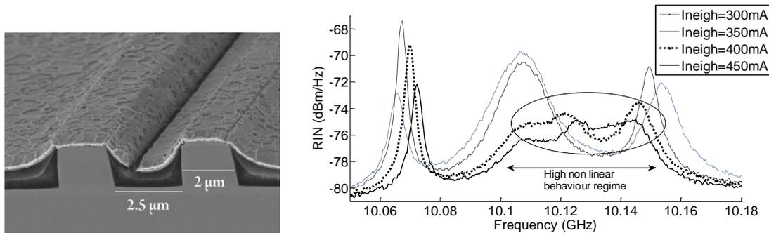
**Figure 1 (right) SEM image of one of the facets of the twin-stripe laser. (left) RIN spectra of the twin stripe laser corresponding to a fixed value for  $I_{\text{main}}$  (400 mA) and 4 values of  $I_{\text{neigh}}$ .**
