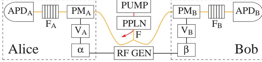
Figure 1: Experimental setup. The PUMP creates photon pairs in the PPLN waveguide and is removed by a filter (F). The photons are manipulated by phase modulators ( $PM_{A,B}$ ), selected by narrowband filters ( $F_{A,B}$ ), and detected by avalanche photo-diodes ( $APD_{A,B}$ ). The phase modulators are driven by a 12.5 GHz radio frequency generator (RF GEN) whose output is controlled by variable attenuators ( $V_{A,B}$ ) and phase shifters ( $\alpha, \beta$ ).
