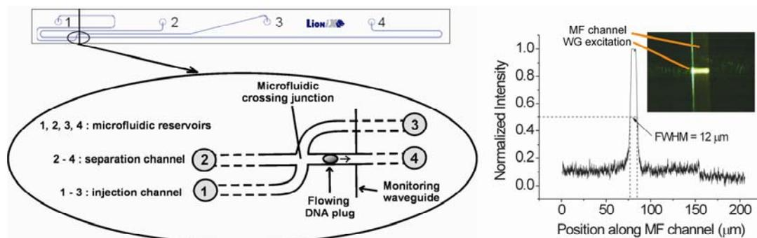
Fig. 1. (a) Layout of the integrated optofluidic chip; (b) integrated WG for localized fluorescence excitation of a MF channel filled with Fluorescein
