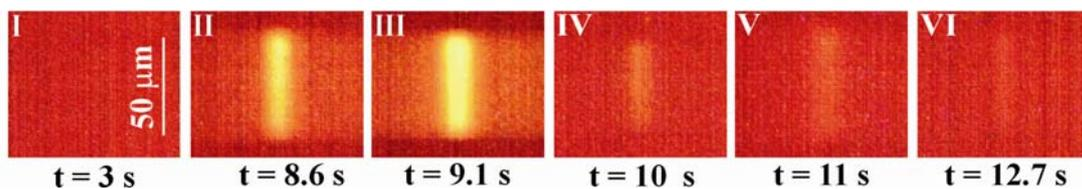
Fig. 2. Fluorescence snapshots of the microchip capillary electrophoresis separation of dsDNA molecules in a MF channel, across an excitation WG, in an optofluidic chip
